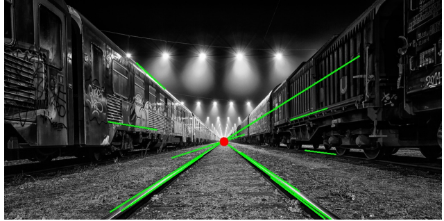
Fig. 12: Result of the vanishing point detection on the image van_points6.jpg
