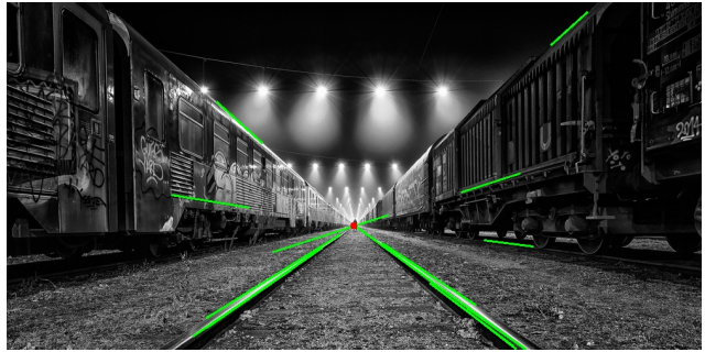
Fig. 10: Result of the vanishing point detection on the image van_points8.jpg
